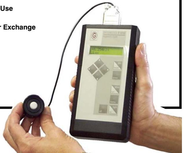
The P-9710 Optometer is a highly efficient single-channel instrument designed for multipurpose use in any photometric and radiometric application.
