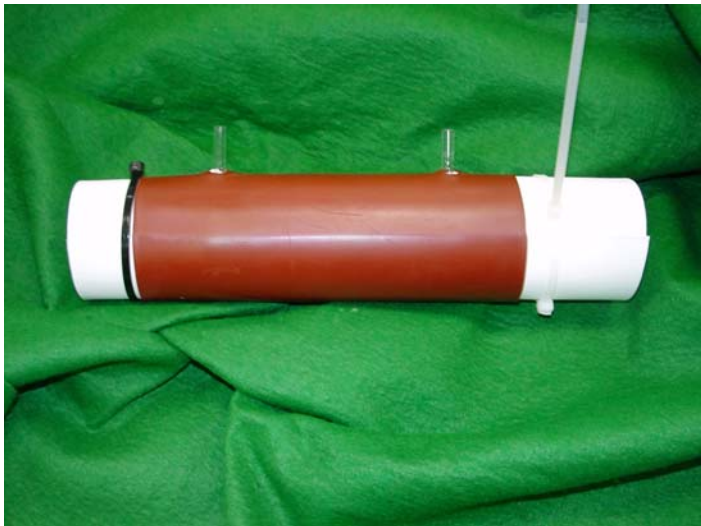
Picture 4: Flow Water Reactor with ODM98 Foil Reflector for Diffuse Light Stimulation
