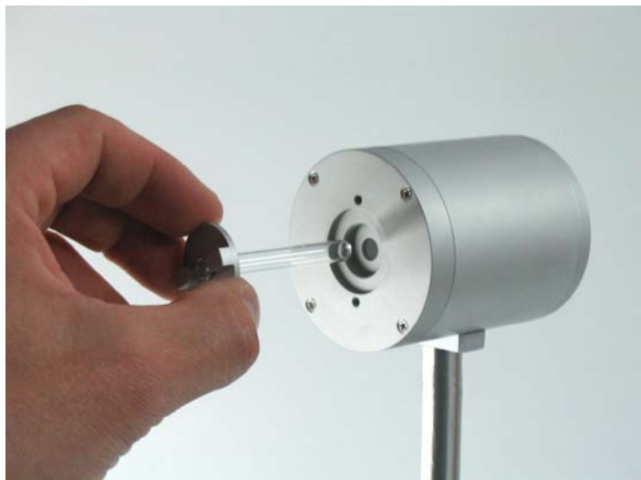
Picture 7: Stretched Integrating Sphere for Side Emitting Fibers with Protection Insert
