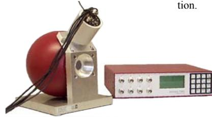
Fig. VI.16. Color and Luminous Flux Measurement Instrument with a 150 mm Integrating Sphere
